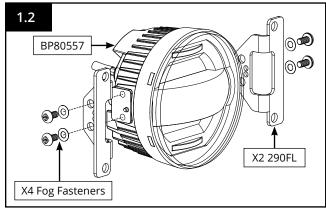
1.3 Using the stich screws provided, mount the fog light to the bar as shown.
